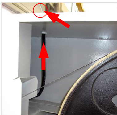
4. Guide the cable through the cable gland.
