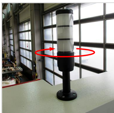
8. Place the signal tower on the base and lock it by turning it briefly in a clockwise direction (see markings on the back of the tower).
